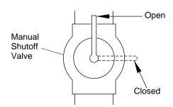
Figure 13 - Manual Shutoff Valve
